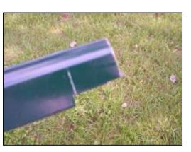
We often make our marks using a square and an awl or similar tool to scratch the finish; a pencil line may be hard to see on dark material. You may notice that the cut is not exactly on the mark; this allows it to be inside the post where it won't be seen.
