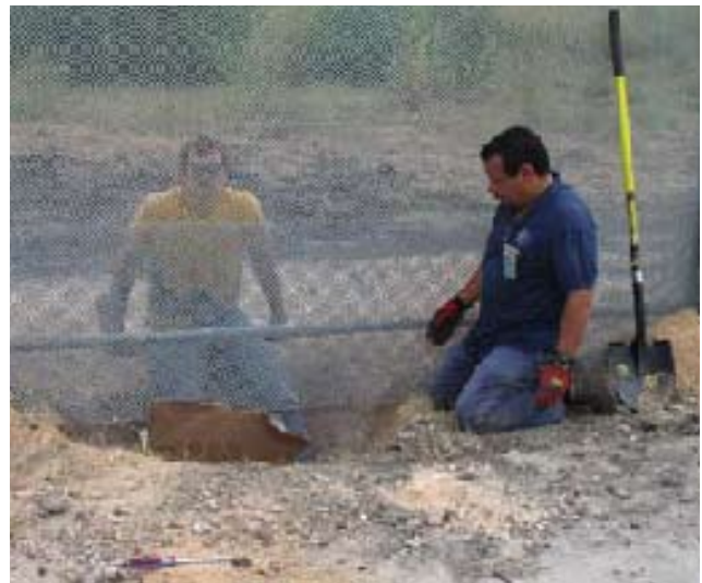
It took 25 minutes for two men with hand tools to dig under a typical buried fence.
