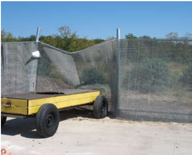
Bogey vehicle weighing 4,000 lbs. and moving 20 mph was stopped in just 4 feet by 1/2" Mesh x 9 GA chain link fence.
