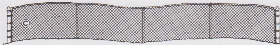
C Fence following grade
