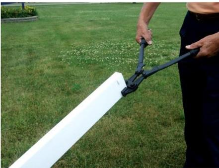
It is often best to invest in a vinyl fence rail remover as shown below. Note the curvature at the end of the metal.
