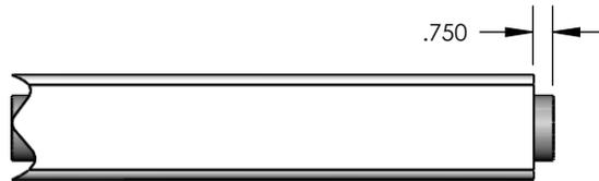
4) Fasten a Mounting Plate to one end of the Aluminum Support Tube using the (4) #10 x 1.000" screws provided. The screws should be installed in between the outside tabs.
