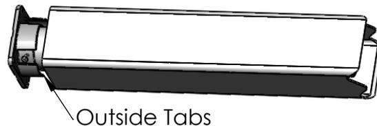
5) Push the Mounting Plate into the exterior PVC Column until it is flush as shown.
